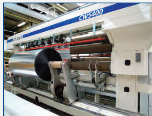
The 4.8m wide Atlas CW5400 Series film slitter under test at Atlas UK prior to shipping
