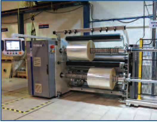
One of the Titan ER610 compact slitter rewinders in action at OPP Film in Lima
