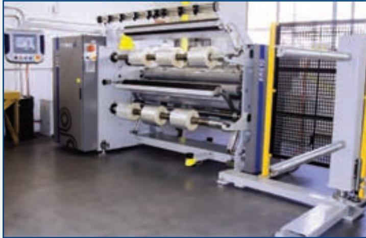
*The Titan ER610 compact slitter rewinder at Plastic Connections, Inc.*
