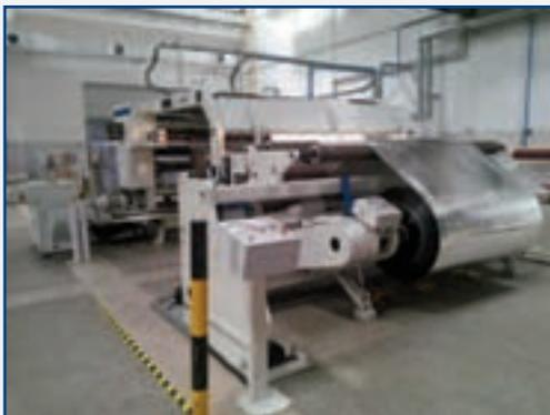
**The 2.5m wide Atlas CW800 secondary slitter for metallized film**
