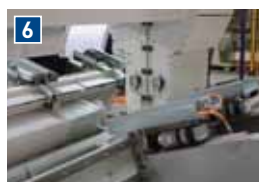
6 Wireless Rewind Arm Positioning Rewind arms are positioned using industrial 'Bluetooth' technology which also sends speed and tension references automatically to the drives. Power is provided by a DC bus bar located under the rewind beams.
