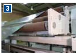
3 Pneumatically Actuated Tension Control The complete assembly moves with edge guide oscillation and linear movement of the roller.
