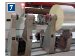
7 Rewind Arms Three types of rewind arms are available for slit widths as narrow as 200mm with heavy-duty arms for wider reels and rewind diameters up to 1200mm (same as primary slitters). A reduced number of belts per driven rewind arm improves reliability. The rewind motors have torque characteristics which increase efficiency & productivity.
