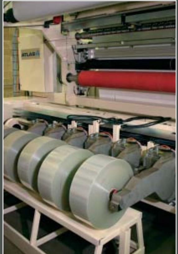
*Slit reels being unloaded automatically on to trolleys*
