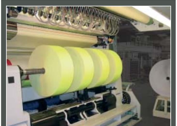
*Internal rewind section of the Atlas OCS-2 slitter rewinder*
