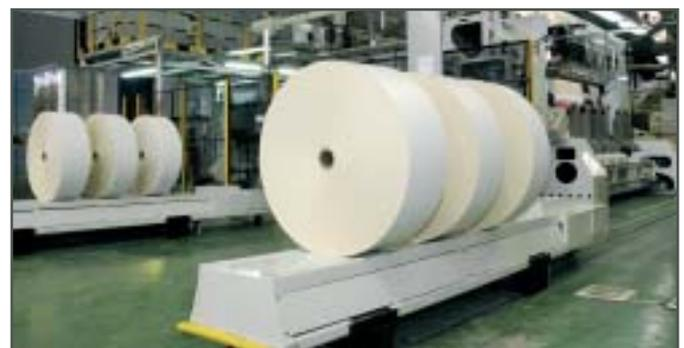
*Labelstock reel transfer on automated trolleys*
