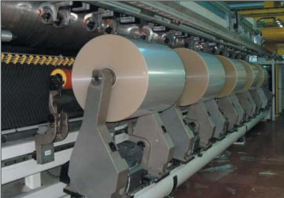
*Atlas is the only company to have supplied 10m wide primary slitter rewinders for BOPP film.*
