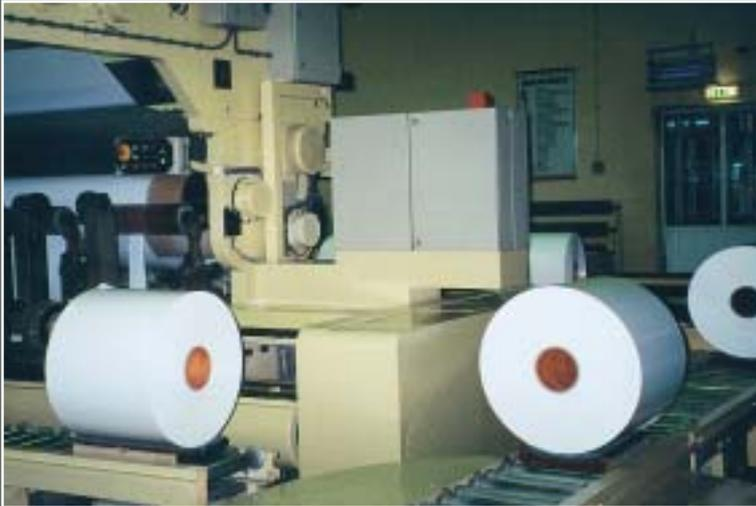
*Finished rolls leaving the slitter via conveyors and turntables*
